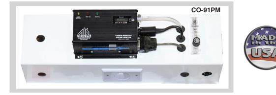
The carbon monoxide (CO) airline monitor panel can be ordered to retrofit any existing Grade-D breathing air system, CO and Oxygen  $(O_2)$  monitor also available. Standard units are supplied with high intensity audible alarm (120 dBA) and a 115 VAC power cord. All units are powder coated steel and ready for wall mounting. Intrinsically safe versions available - CSA approved, 9 VDC power only. **Supplied Grade-D air filtration is required to operate the monitor**.
